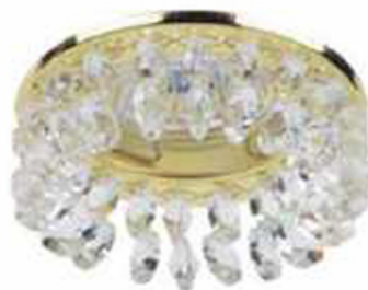
HX-A8076 HOLDER-POWER: MR16-50W SURFACE MATERIAL: IRON+CRYSTAL LAMP SIZE-mm: Φ81*60 CUT-mm: Φ65
