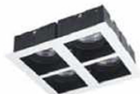
HX946-4S COLOUR: WH HOLDER: 4xGS.3(MR16) SURFACE MATERIAL: IRON LAMP SIZE-mm: L168xW157xH45 CUT-mm: L160xW140
