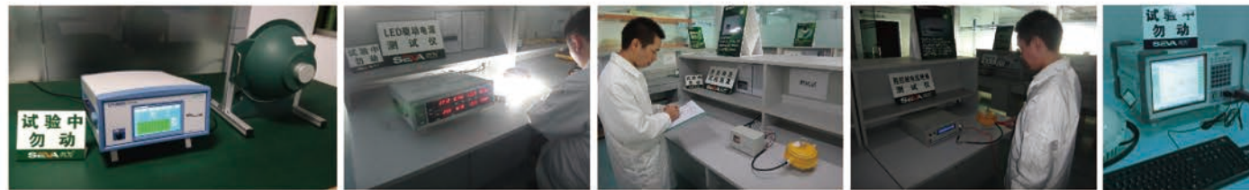
⑱Light source stroboscopic test system ⑲LED driver test ⑳Switch impact test ㉑Withstanding insulation voltage test ㉒Volt insulation test
