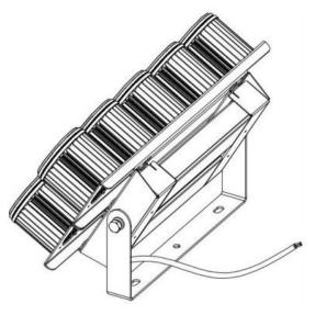
ACL: Connect the Brown input ACN: Connect the Blue input
